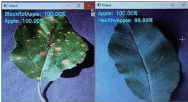
Fig. 9 Result of detection and recognition of an apple plant with 100% accuracy and shows a leaf infected with a black rot disease on the left image and a healthy leaf on the right image.
